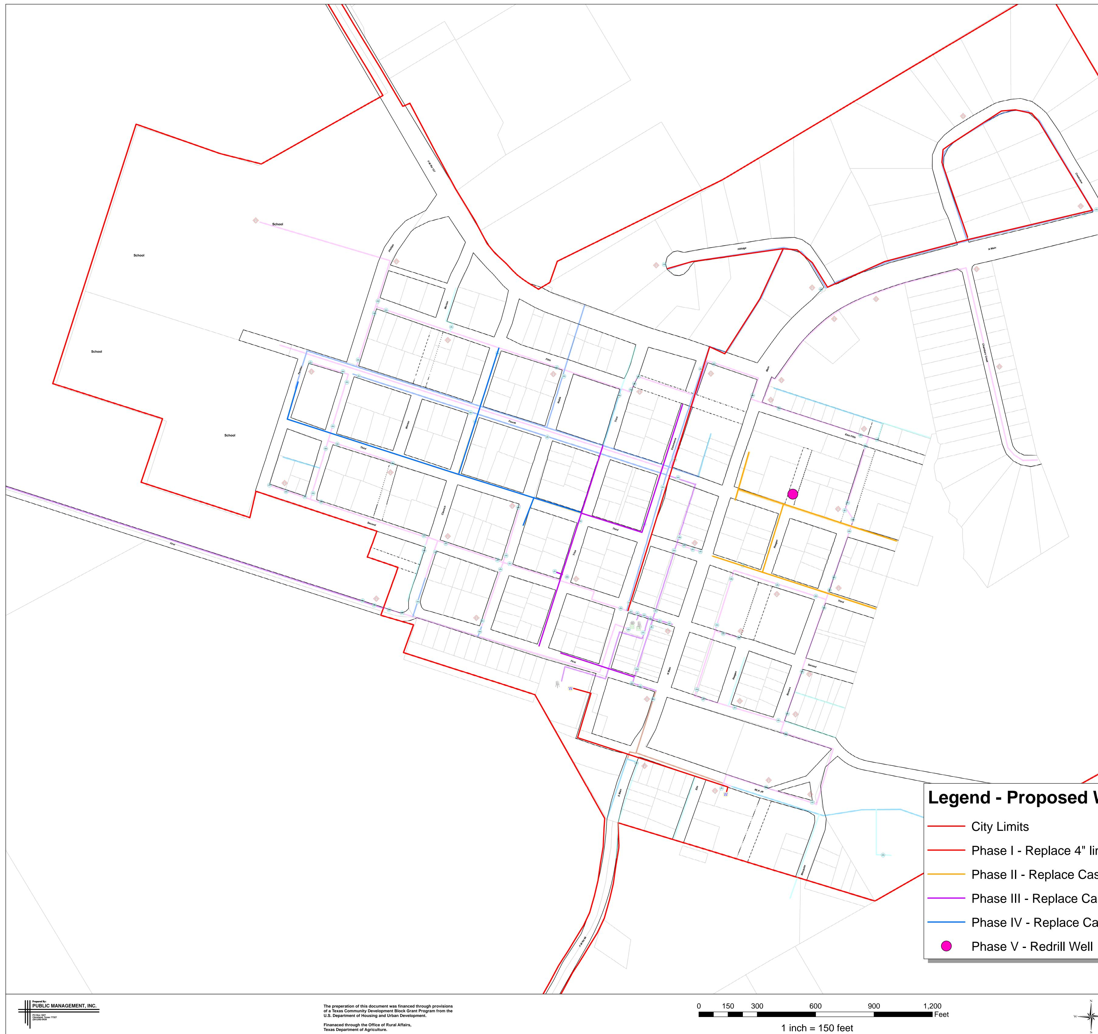
Legend - Proposed Water Improvements Phase I - Replace 4" lines with 6" lines; Connect Well #2 to Well #4 Phase II - Replace Cast iron Lines with PVC lines Phase III - Replace Cast iron lines with PVC lines Phase IV - Replace Cast iron lines with PVC lines
